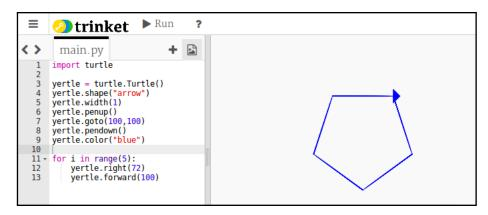
**Fig. 12:** *Drawing generated by drawing the sequence* 100, 100, 100, ... *with grid rotations of* 72 *degrees.*
