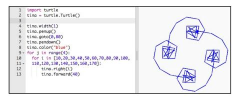
Fig. 13: Python code (left) and drawing (right) generated by a sequence of angle measures.
