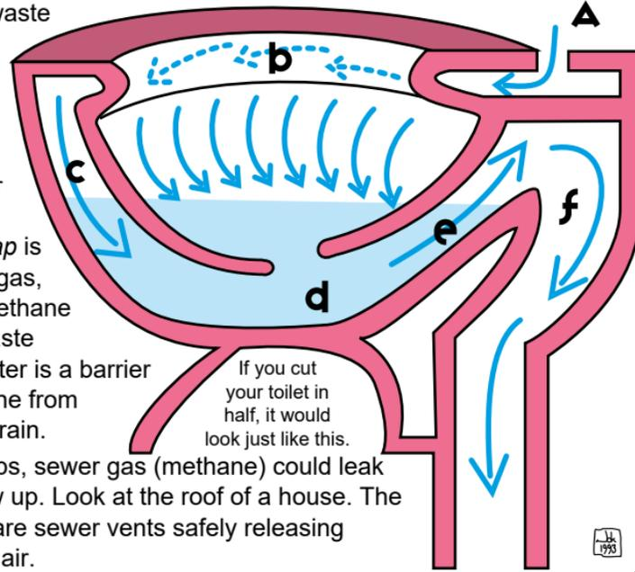
There is always water in the trap (E). The reason it's called a *trap* is that it traps methane gas, which is explosive. Methane gas is made when waste decomposes. The water is a barrier that keeps the methane from coming back up the drain. Before drains had traps, sewer gas (methane) could leak into a house and blow up. Look at the roof of a house. The black pipes up there are sewer vents safely releasing methane gas into the air.
