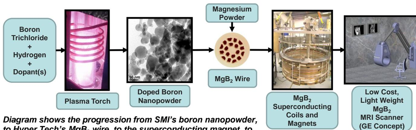
*Diagram shows the progression from SMI's boron nanopowder, to Hyper Tech's  $MgB_2$  wire, to the superconducting magnet, to a low cost, light weight MRI scanner*
