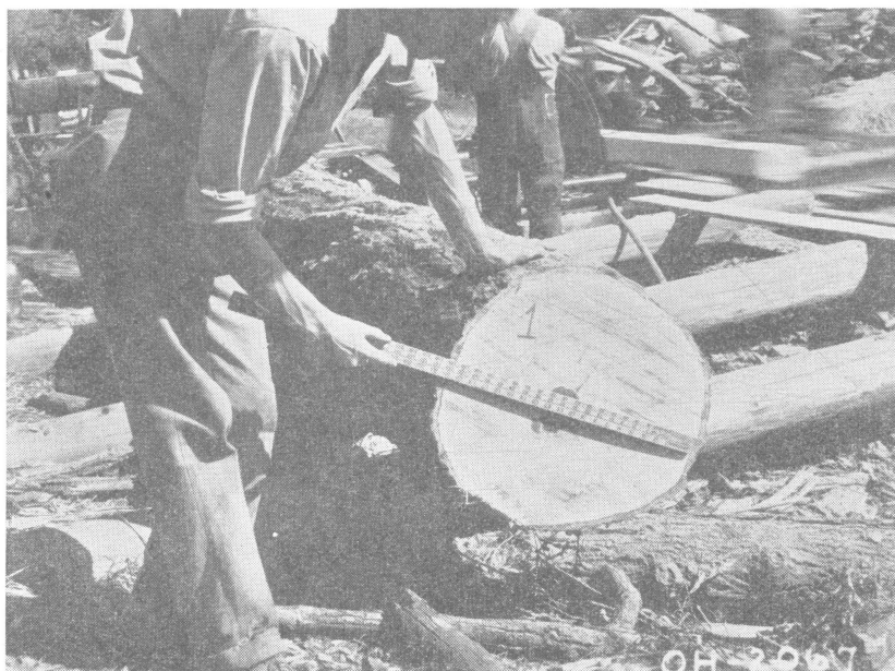
Fig. 16. Scaling an oak log on the log deck of a portable mill. Both the long and short diameters are read and averaged to get the log diameter. Note the center rot which must be scaled out.
